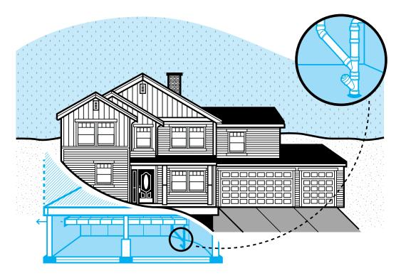
BECAUSE THEY'RE UNVENTED, SEALED CRAWLSPACES REQUIRE A TERMINAL THAT BRINGS IN CONDITIONED AIR.
