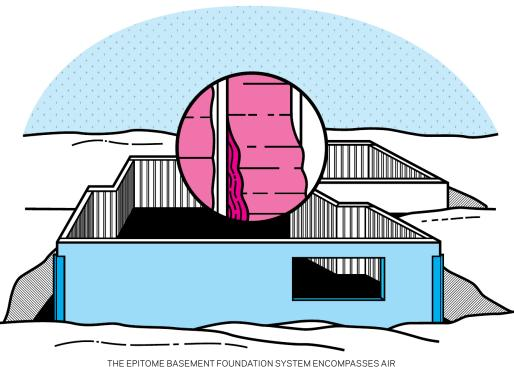
HE EPITOME BASEMENT FOUNDATION SYSTEM ENCOMPASSES A AND MOISTURE BARRIERS AND INSULATION.
